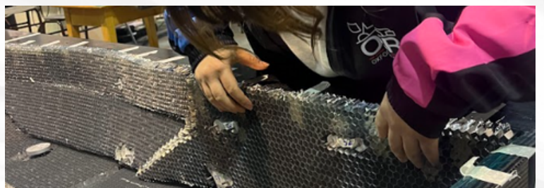
Ume placing Corex honeycomb core in the chassis
